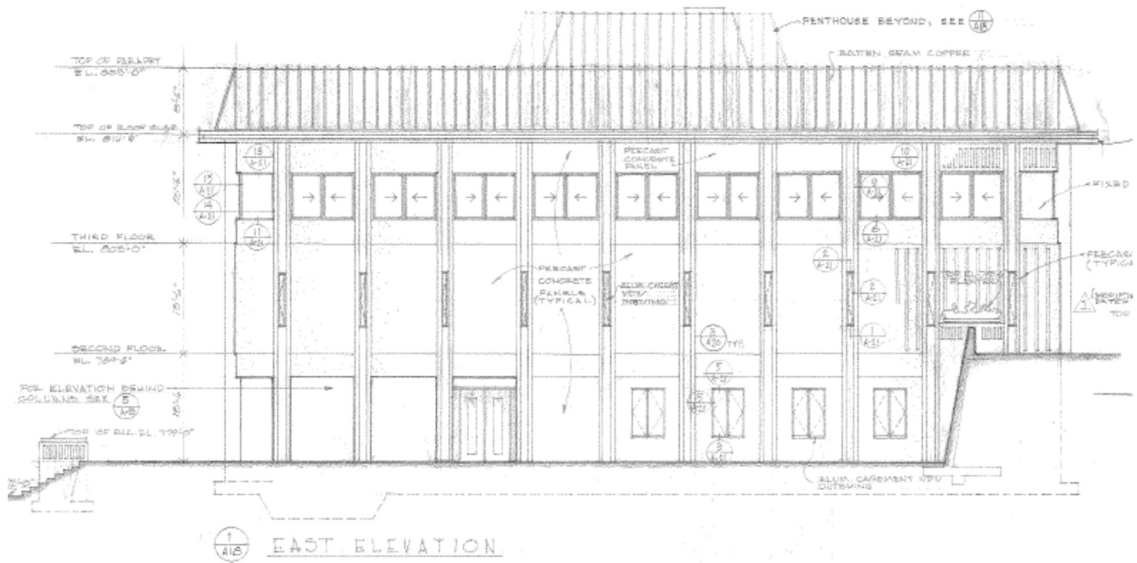
East elevation from original structural drawings
